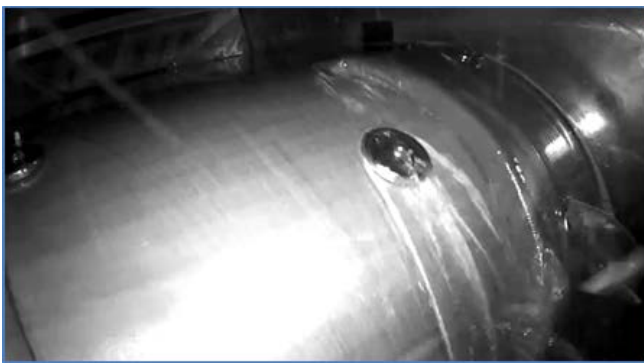
Photo 2. Lamprey successfully passing the radius curve on April 30, 2017 (1st night after the round magnets were added) (left photo). Strategically placed magnets effectively break up the flow and allow lamprey to choose the best path for their passage based on their preferred flow conditions (right photo shows the view from the top with multiple lamprey climbing the center with a flow break created by the magnets).
